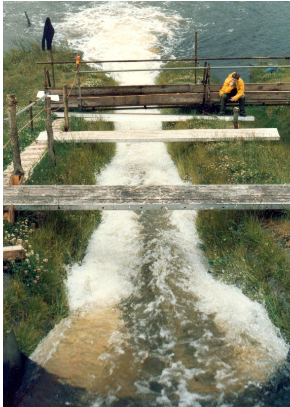
GRASSCRETE under test with tail water observation
